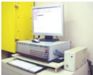
Rackmount multi SRO Modbus with 10 wells integrated.
