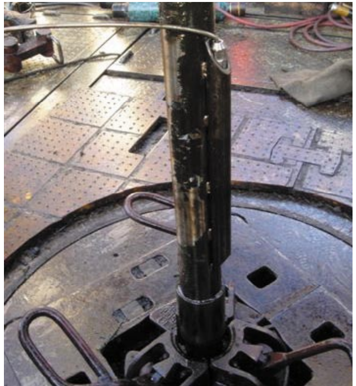
Welded Carrier with secured Continuous Monitoring Tool and Cablehead attached to tubewire.
